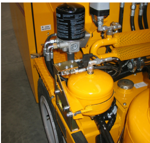
Air drier for bead tank
