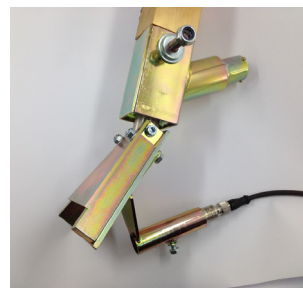
Bead alarm mounted on bead gun
