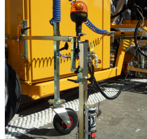
Pre-marking system with paint can
