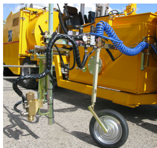
Pre-marking system with paint gun
