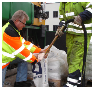
Ejector filling of bead tank
