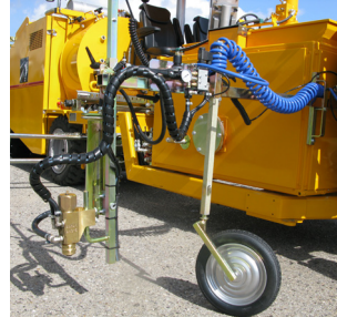
Pre-marking system with paint gun
