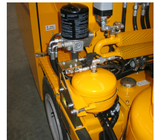
Air drier for bead tank
