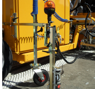
Pre-marking system with paint can
