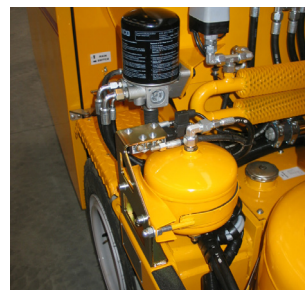
Air drier for bead tank
