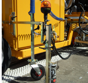
Pre-marking system with paint can
