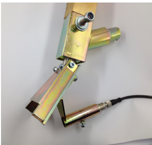
Bead alarm mounted on bead gun
