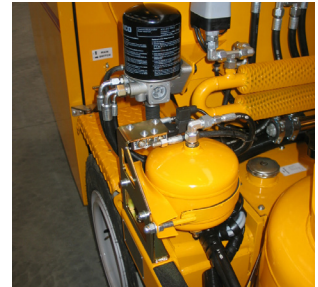
Air drier for bead tank
