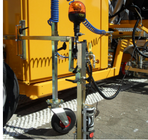
Pre-marking system with paint can
