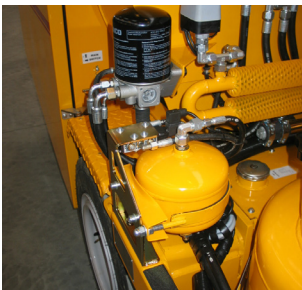
Air drier for bead tank
