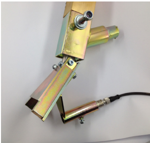
Bead alarm mounted on bead gun
