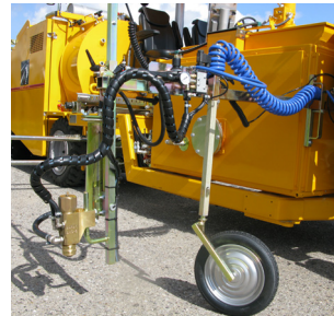
Pre-marking system with paint gun
