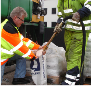
Ejector filling of bead tank
