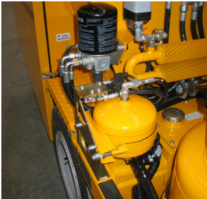
Air drier for bead tank
