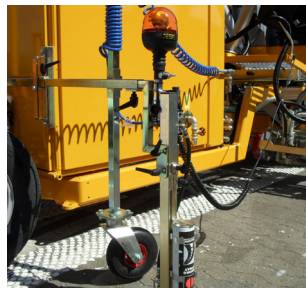
Pre-marking system with paint can
