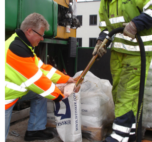
Ejector filling of bead tank
