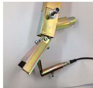
Bead alarm mounted on bead gun
