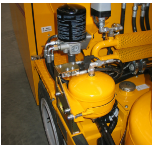
Air drier for bead tank
