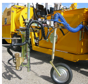
Pre-marking system with paint gun
