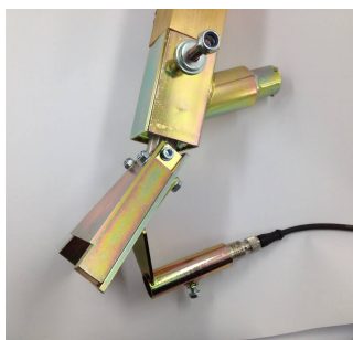
Bead alarm mounted on bead gun
