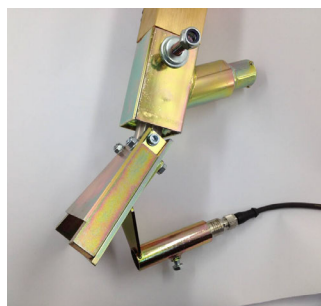
Bead alarm mounted on bead gun
