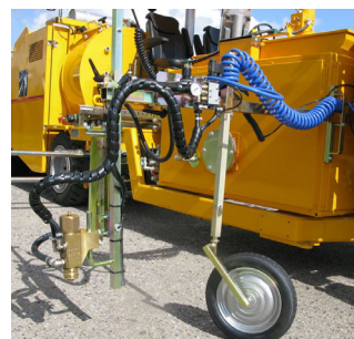
Pre-marking system with paint gun
