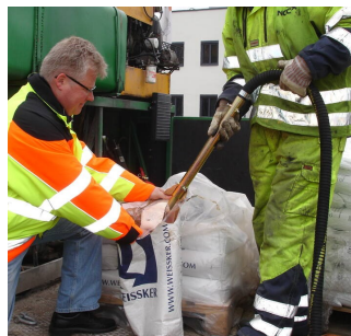
Ejector filling of bead tank
