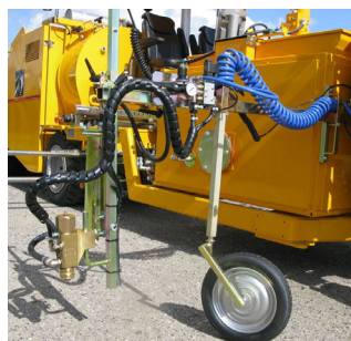
Pre-marking system with paint gun
