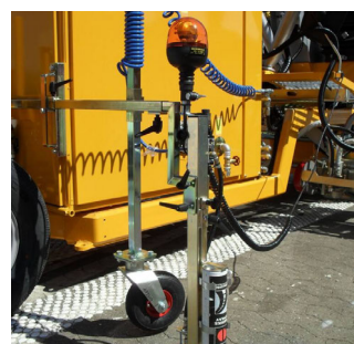
Pre-marking system with paint can
