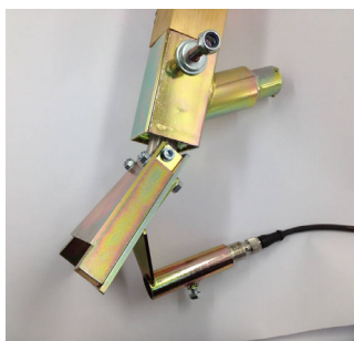
Bead alarm mounted on bead gun
