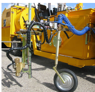
Pre-marking system with paint gun
