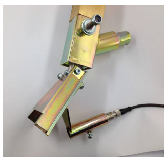
Bead alarm mounted on bead gun
