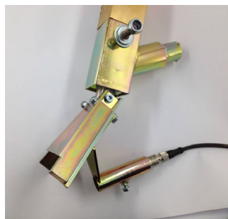
Bead alarm mounted on bead gun
