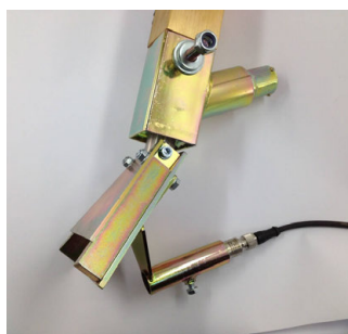
Bead alarm mounted on bead gun
