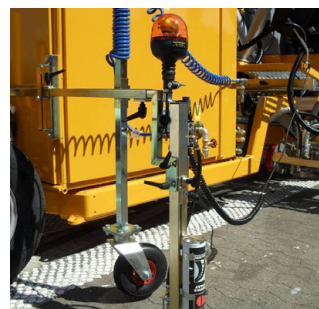
Pre-marking system with paint can
