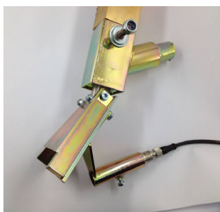
Bead alarm mounted on bead gun
