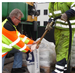
Ejector filling of bead tank
