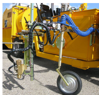
Pre-marking system with paint gun
