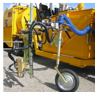
Pre-marking system with paint gun
