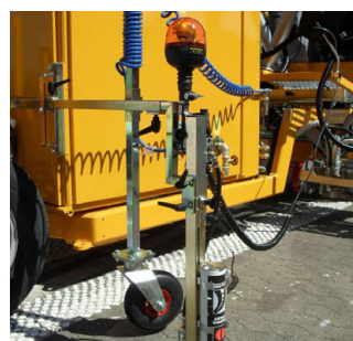
Pre-marking system with paint can
