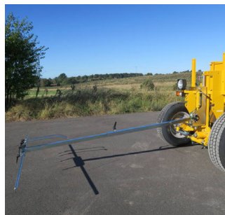
Pointer turning with steering
