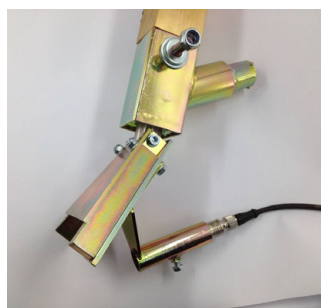
Bead alarm mounted on bead gun
