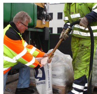
Ejector filling of bead tank
