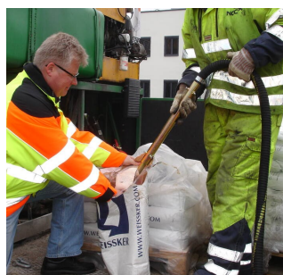
Ejector filling of bead tank
