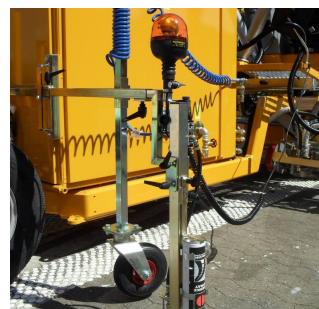
Pre-marking system with paint can
