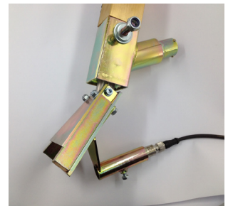
Bead alarm mounted on bead gun
