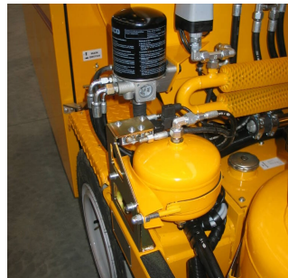
Air drier for bead tank
