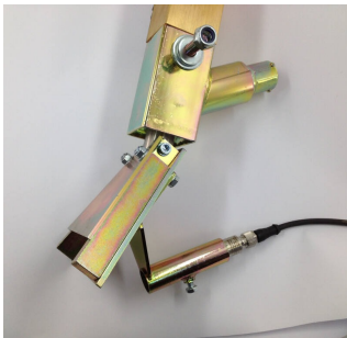
Bead alarm mounted on bead gun
