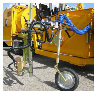
Pre-marking system with paint gun
