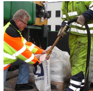
Ejector filling of bead tank
