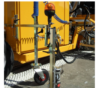
Pre-marking system with paint can
