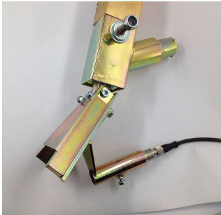
Bead alarm mounted on bead gun
