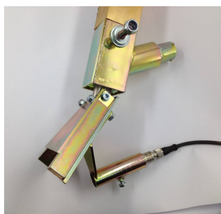
Bead alarm mounted on bead gun
