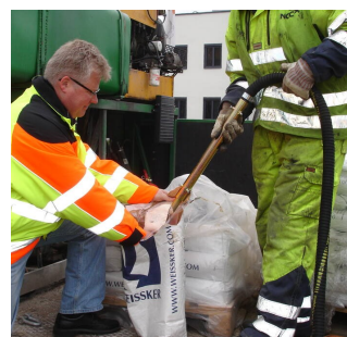
Ejector filling of bead tank
