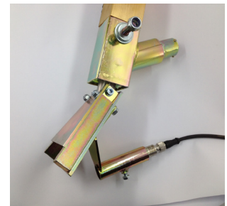
Bead alarm mounted on bead gun
