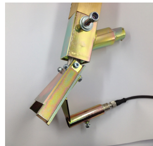
Bead alarm mounted on bead gun
