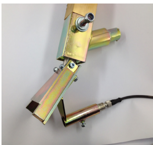
Bead alarm mounted on bead gun
