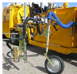
Pre-marking system with paint gun
