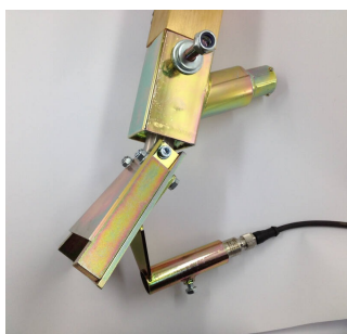
Bead alarm mounted on bead gun
