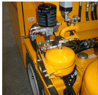
Air drier for bead tank
