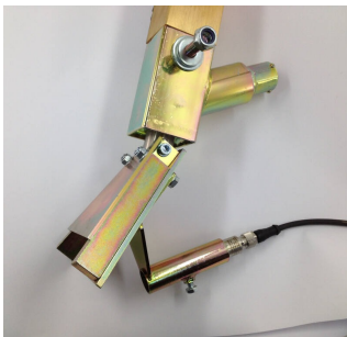
Bead alarm mounted on bead gun
