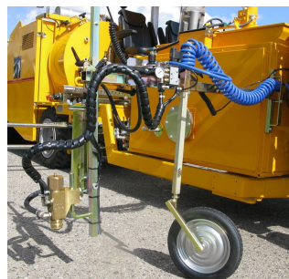
Pre-marking system with paint gun
