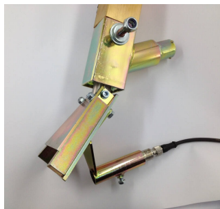
Bead alarm mounted on bead gun
